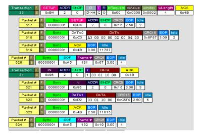
When you instruct the Analyzer to display USB transactions, the components of each transaction are collected from the current recording and are grouped and indented below each decoded transaction. Each row shows a transaction with a unique numeration, a label, and color-coded decoding of important data.
