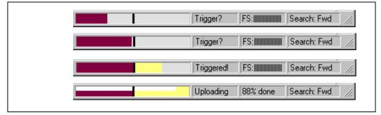
As recording progresses, the Progress Indicator changes to reflect the recording progress graphically:
