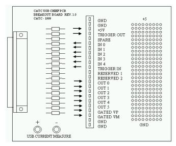
The External Interface Breakout Board is an accessory that allows convenient access to several potentially useful TTL output and input signals. It also offers a simple way to connect logic analyzers or other tools to the Analyzer unit.
