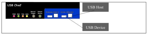
The **Record & Generate** port has both type 'A' and type 'B' connectors so the Analyzer can conveniently tap a USB branch. To connect your USB branch for analysis, use the two **SHORT** (3-foot/1-meter) USB cables to insert the Analyzer in place of the existing cable. Connect one cable to the type 'A' connector and join it downstream to your device or hub. Connect the other cable to the type 'B' connector and join it upstream to your host or hub.
